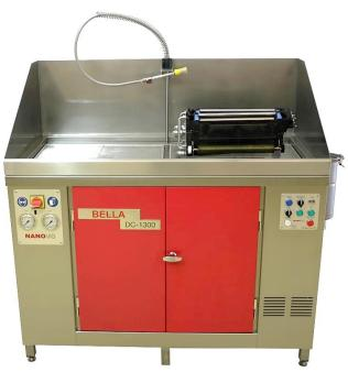
Ink tanks, application rollers, etc. are cleaned efficiently and sustainably with the HP specific Imaging Oil. The highlight is the integrated recycling system, which continuously removes ink particles from the Imaging Oil. This has the advantage that the dirty parts are always cleaned with a consistently clean Imaging Oil. This reduces operating costs and the volume of hazardous waste to a minimum.
